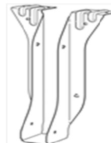
FIGURE 1c—JBA HANGER (LBAZ HANGER SIMILAR)
